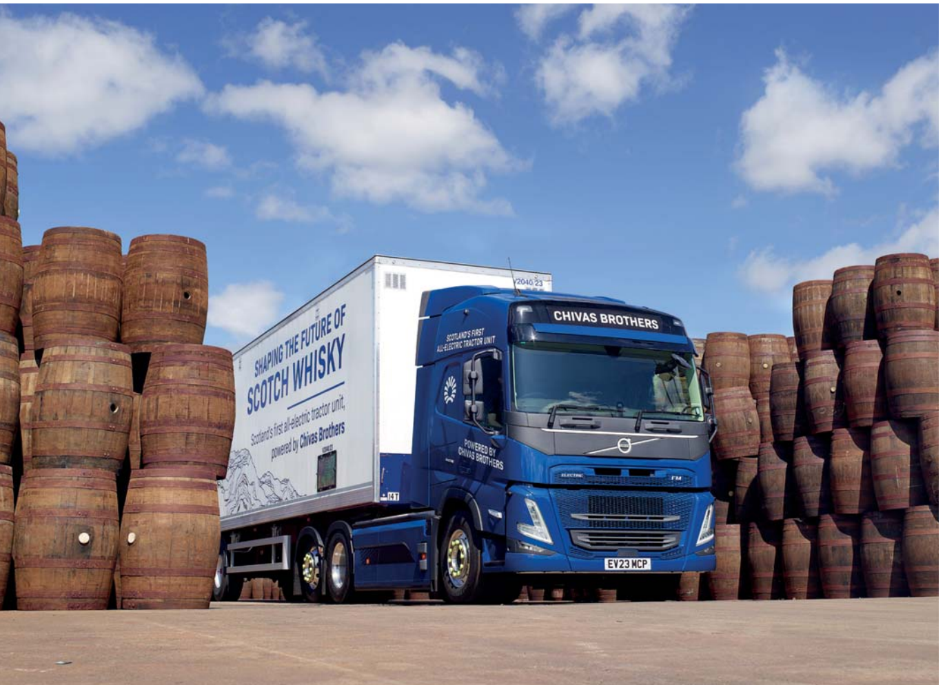
Smooth yet powerful: Scottish distillery Chivas Brothers has employed a 6x2 44-tonne FM Electric with a range of up to 250km
