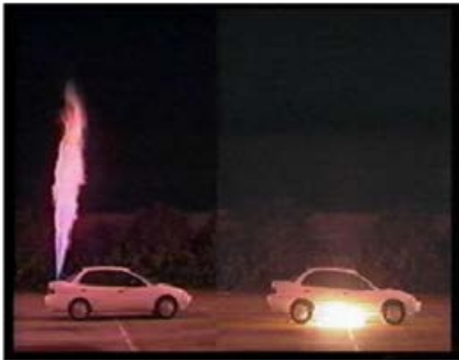
Photo 2 - Time 0 min, 3 seconds - Ignition of both fuels occur. Hydrogen flow rate 2100 SCFM. Gasoline flow rate 680 cc/min.
